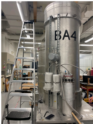
BA 220/270 GHz receiver, currently at Stanford.
