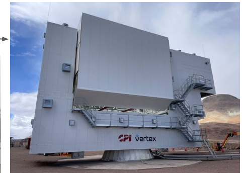
Ongoing fabrication of prototype mirror test stand
