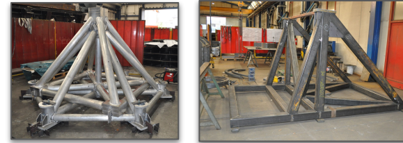
Ongoing fabrication of prototype mirror test stand
