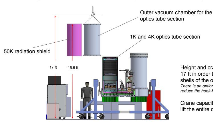
Height and crane requirement: 17 ft in order to install the outer shells of the optics tube section. There is an option to modify the cart and
