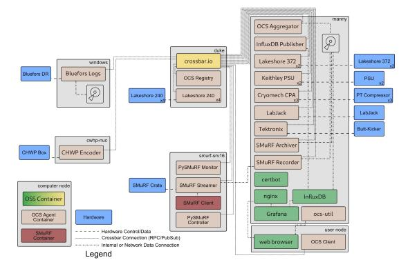
(Example from a SAT testbed at UCSD)
