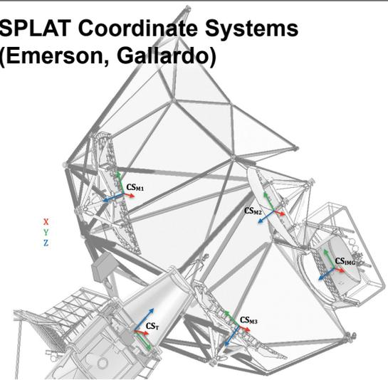
Figure 5 - Mirror and image plane coordinate systems
