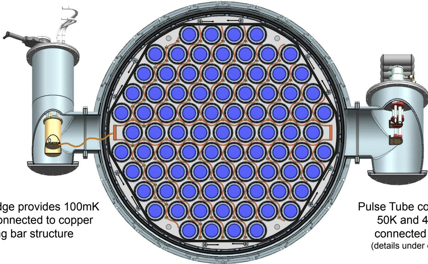
Dilution fridge provides 100mK cooling connected to copper cooling bar structure
