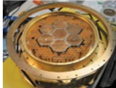
SPTpol focal plane • 2012 - 2016 • 1,600 bolometers • 95/150 GHz • Pol. sensitive
