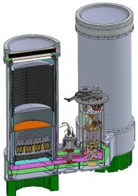
Cutaway of individual optical tube and common dilution refrigerator.
