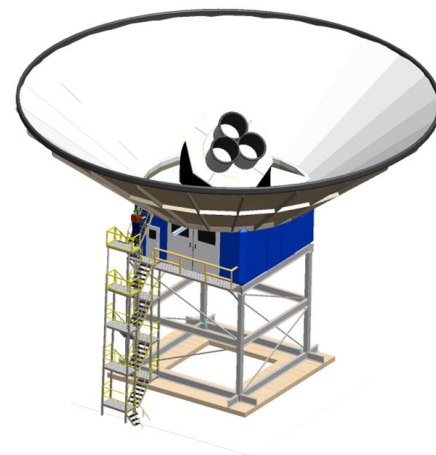
S4 SATs mount and groundshield (total 6 planned)
