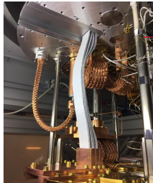
300K-to-4K and 4K-to-100mK cabling and heatsinks
