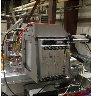
MCE readout electronics built by UBC used in prototyping and to start test stands
