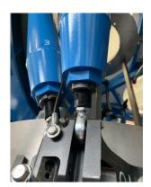
Ex: Mount-Receiver Strut Interface from BICEP Array
