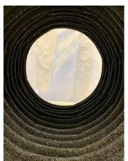
HR-10-coated baffle rings in 4K optics tube suppress sidelobes measured in previous BICEP receivers **Simons Observatory**
