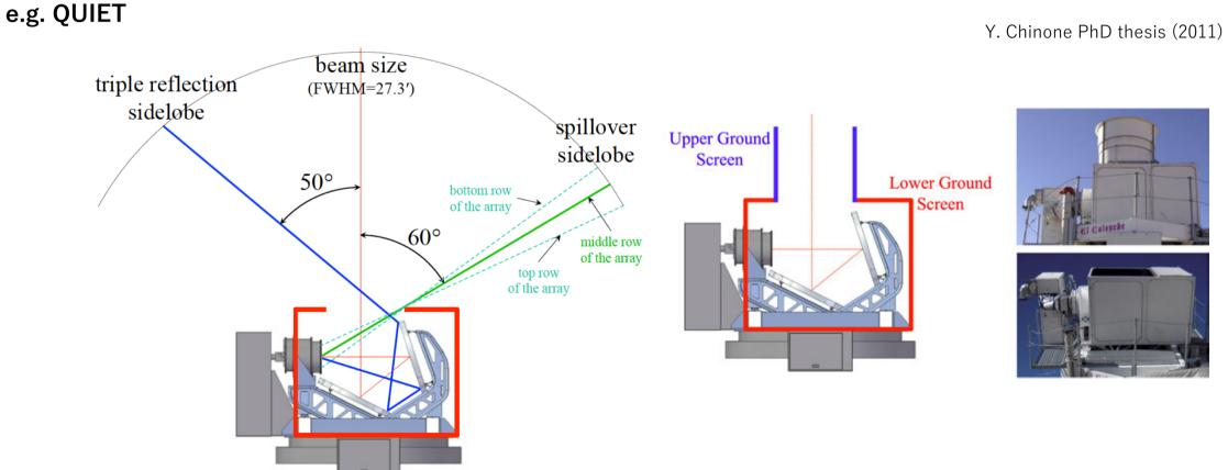
With simulation and measurement, we knew the upper-ground screen is important to prevent SSS. But deployment of the upper-ground screen was delayed. We started observation w/o it.
