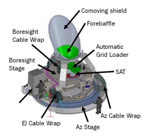
For SO SAT, a forebaffle and comoving shield (and ground screen) have been designed and will be deployed before observation.
