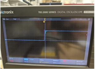
Boundary clock and Grandmaster aligned to 16ns (fluctuates within 100ns spec)
