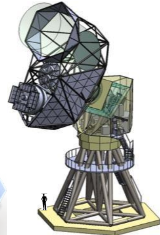
5m TMA design with monolithic mirrors and boresight rotation at South Pole
